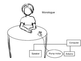
Connect the computer to the Arduino uno, convert the audio output signal into an electrical signal, and drive the motor-pump to play the heartbeat tempo at the same time. P.S. The equipment can be placed under the table and covered by clothes
